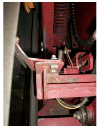
Dismantle original inferior chain slider in order to modify its front part as shown in this picture.
